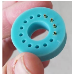
PMT socket produced in FABLAB ULS
