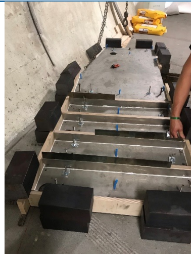
Survey and positioning of baseplates for muon filters
