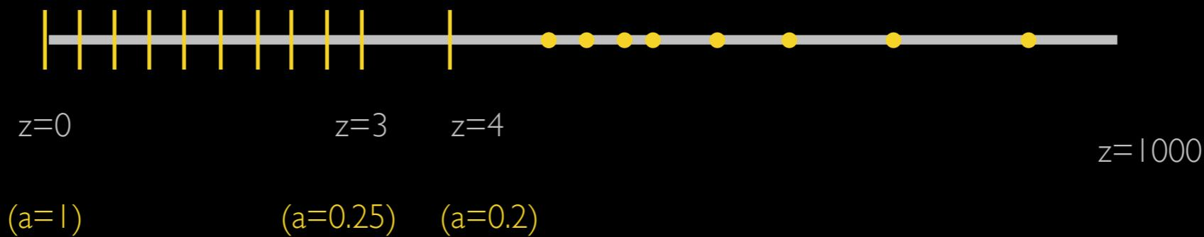
The three functions are represented by their values at **11 discrete** values (**nodes**) of  $a$ , with a **cubic spline** used to interpolate between them.
