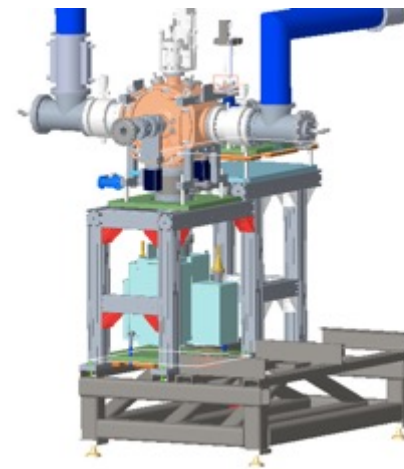
Rendering of new 500 Cu bunching cavity for CeC accelerator
