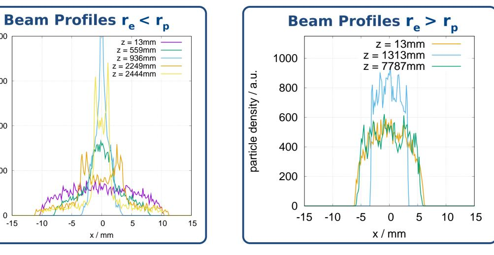
The radii of the beams are varied. In the case that  $r_e < r_p$ , non-linear fields arise, which leads to a periodic change of the distribution and possible losses. In the case that  $r_e > r_p$ , the distribution is preserved. If the density difference of the beams is small, then only a periodic compression and decompression occur.
