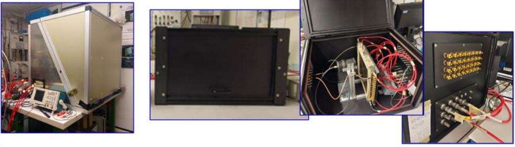
Initial dark-box; then, optimized dark-box modified to improve light-tightness and operative needs
