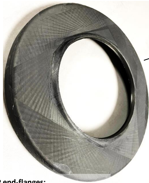
CFRP end-flanges: Complex geometries to design interfaces with end-plates, feedthroughs, detector, magnet, ... in future cryostat.
