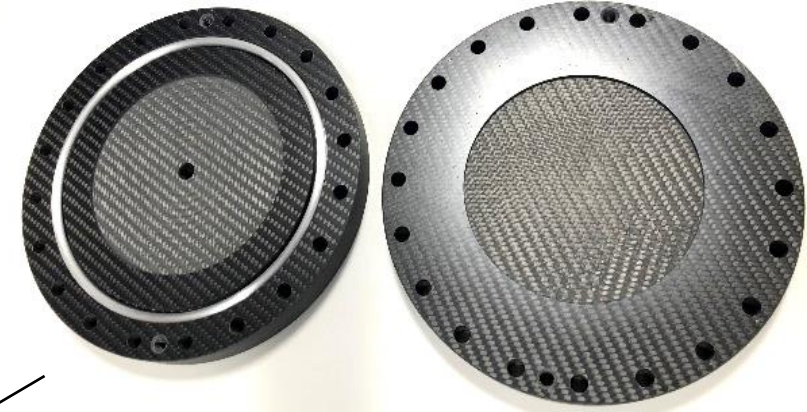
CFRP-sandwich end-plates: Dismountable joint sealed with Helicoflex seal (UHV standard)
