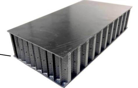
-Full Carbon Sandwich for Cryo temperature
