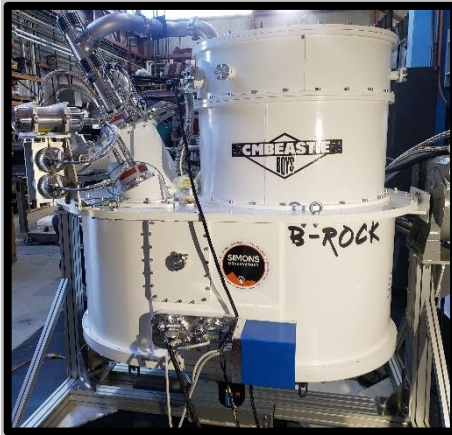
Nr. 3 Cryostats for Simons Observatory telescope (San Diego University, CA)
