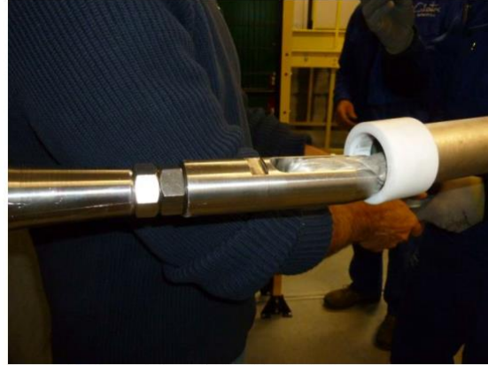
Figure 4.b) the cable entering the jacket
