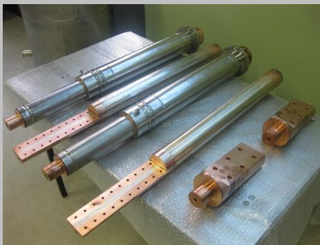
Design and manufacturing of 20 KA current leads, suitable to work with two cooling fluids (LHe and LN2) or at 10 KA with LHe only
