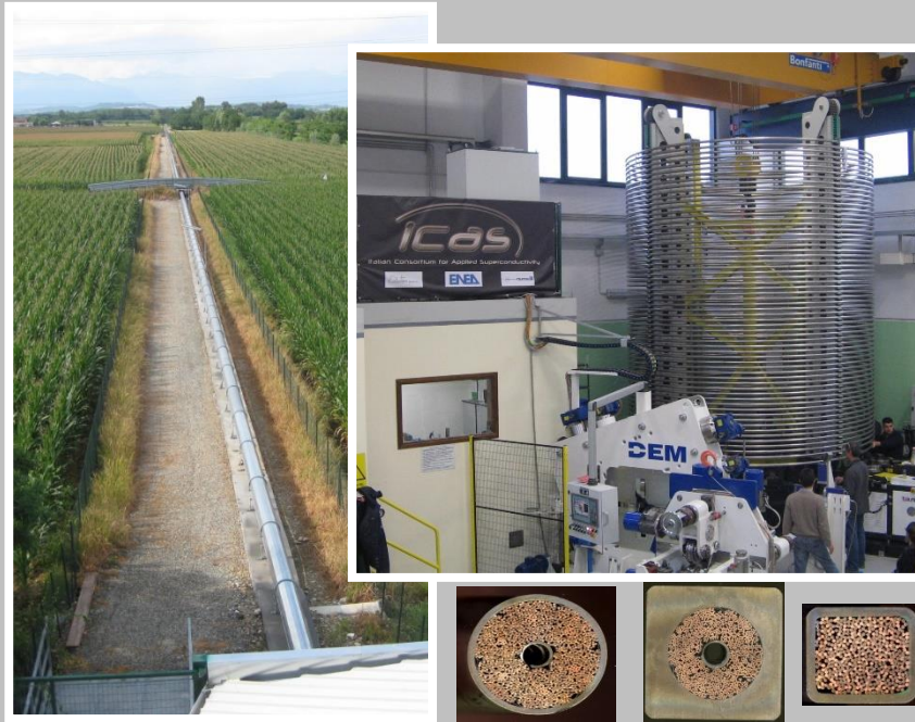
Jacketing line for the production of CICC conductors for ITER project
