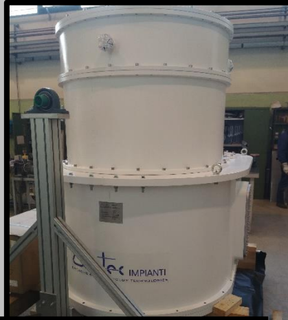
Nr. 3 Cryostats for Simons Observatory telescope (San Diego University, CA)
