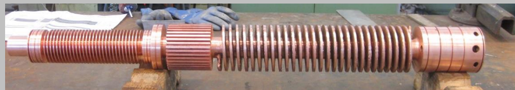
Design and manufacturing of 20 KA current leads, suitable to work with two cooling fluids (LHe and LN2) or at 10 KA with LHe only
