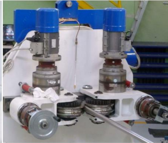
Fig2. B. Third roller pair at the compaction machine exit
