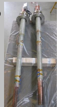
Design and manufacturing of 20 KA current leads, suitable to work with two cooling fluids (LHe and LN2) or at 10 KA with LHe only
