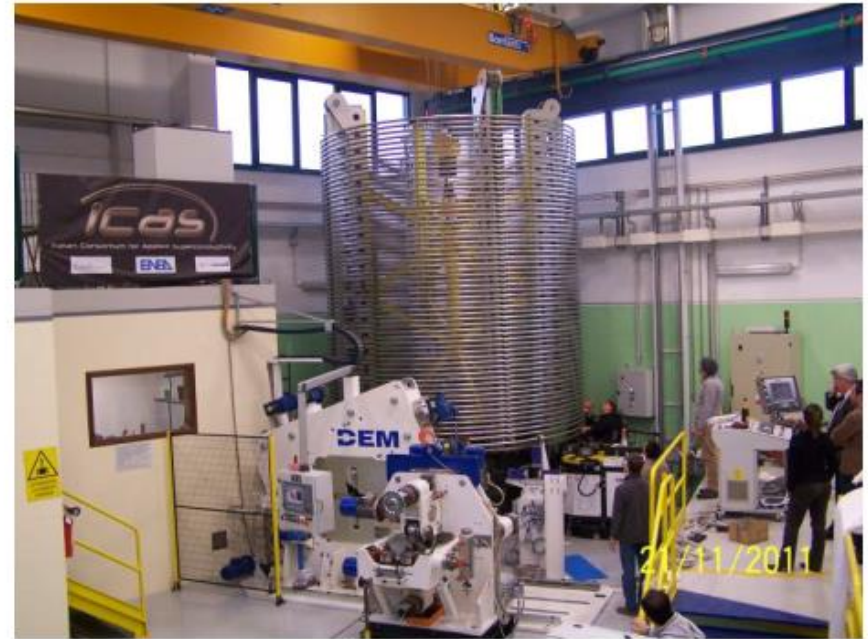
Fig.7 a. spooled ITER TF Cu dummy conductor
