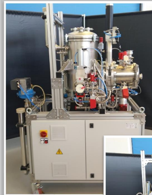
Offgassing test chamber (Thales Alenia Space Italy)
