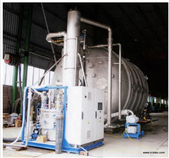
Satellite test facility (5 mt wide, 5 mt long, with cryogenic cooling system at 80 K)
