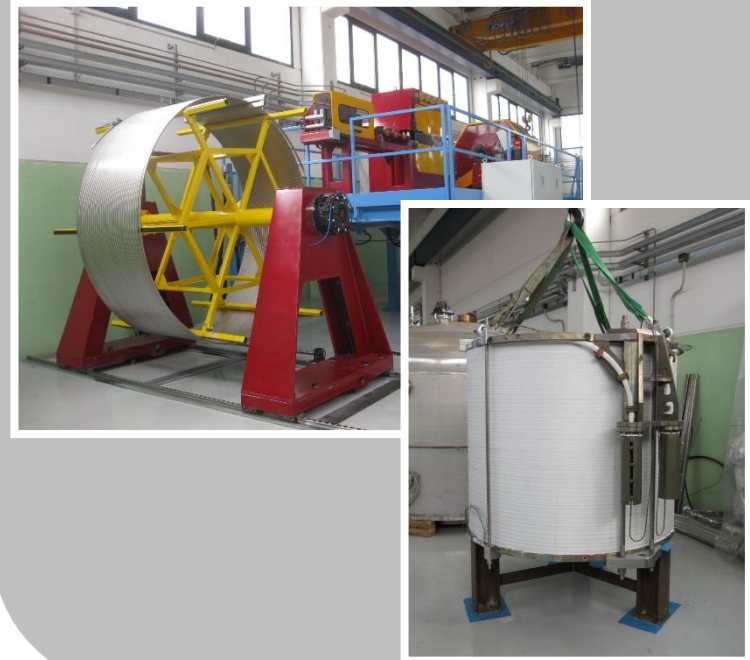
Winding line for the manufacturing of Superconducting magnets.
