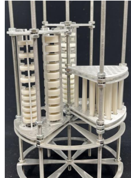
Aluminium cradle for irradiation test campaign
