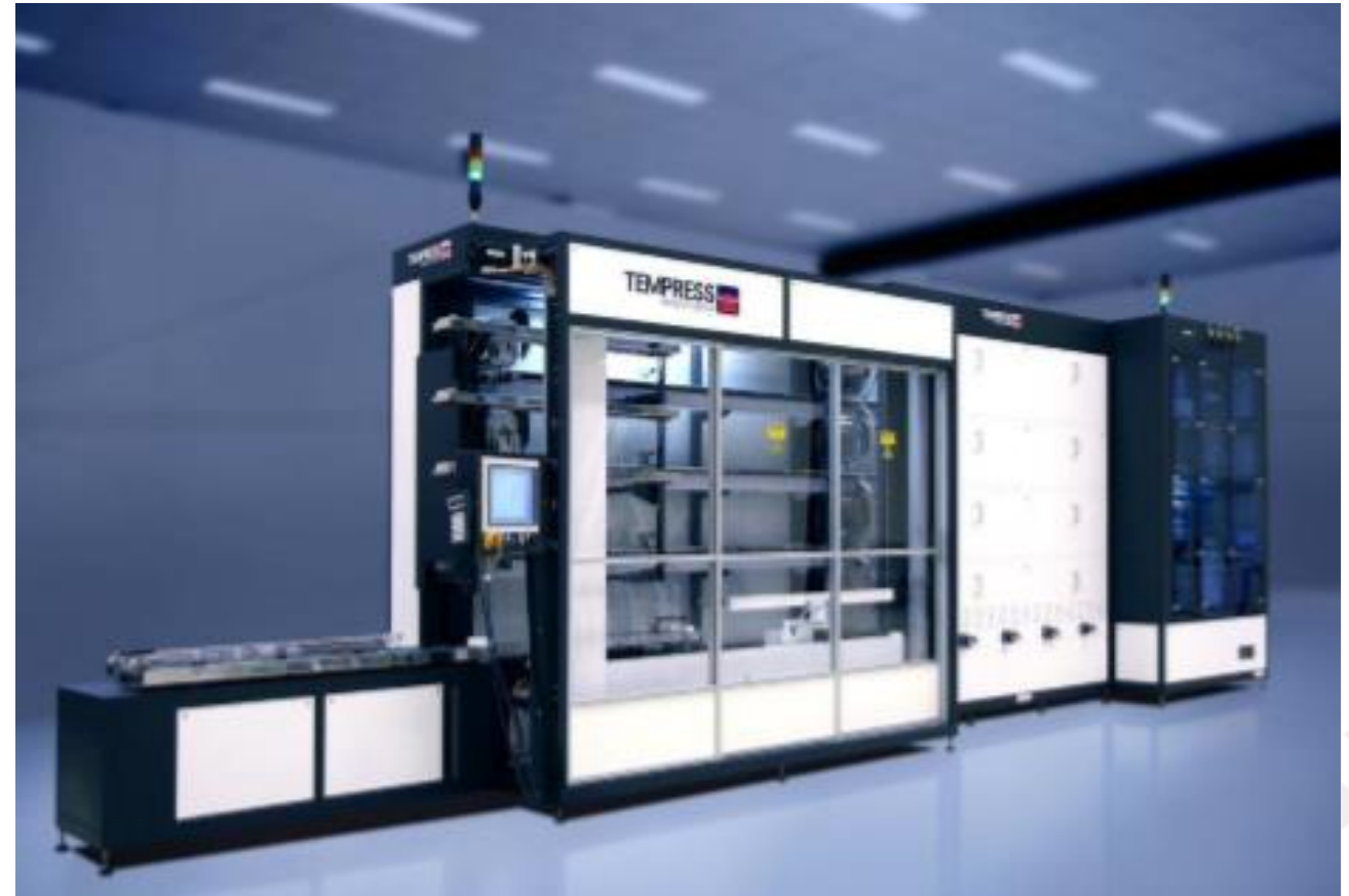
New furnaces, 12 tubes, atmospheric and low pressure
