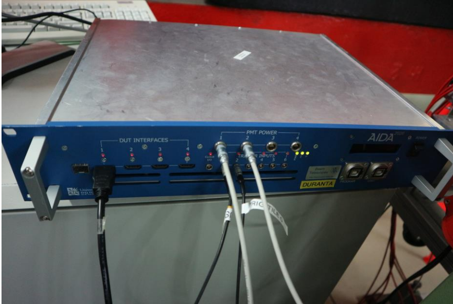
AIDA-2020 TLU connected to beam telescope
