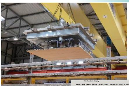
Vertical Drift Charge Readout Planes (CRPs) with perforated anodes have been successfully constructed and tested at the CERN Neutrino Platform
