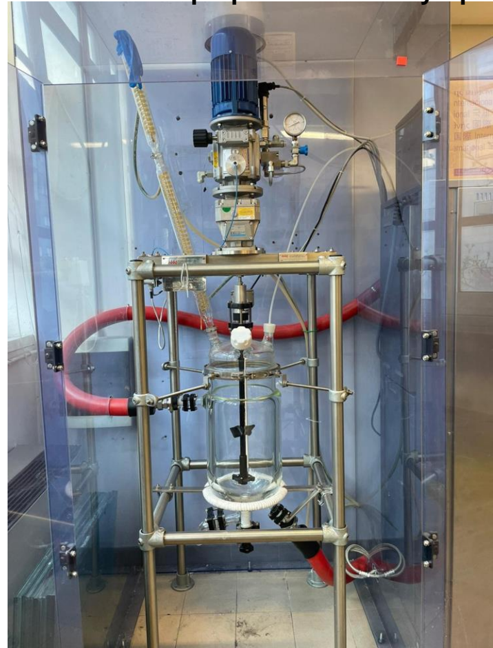
The reactor to prepare the MMA syrup
