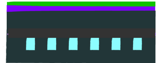
Monolithic CMOS detector with integrated micro-channels
