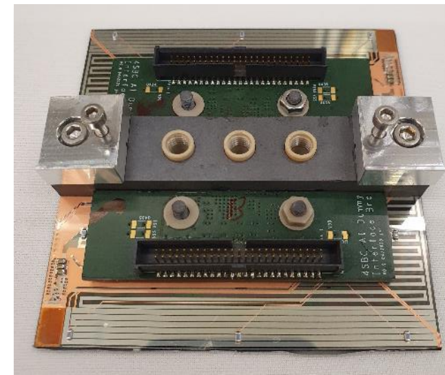
Interface PCB and Bracket connectors assembled
