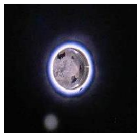
Inlets/outlet open By Laser drilling
