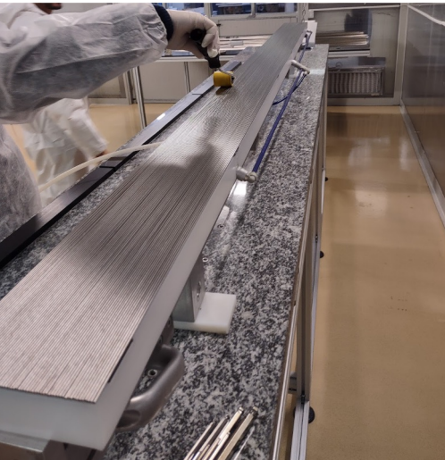
Glue dispensing and tube alignment and positioning
