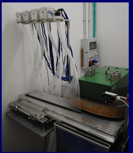
Scintillating fiber detector for electron spectrometer (laser-plasma acceleration experiment PLASMONX), now working in Frascati
