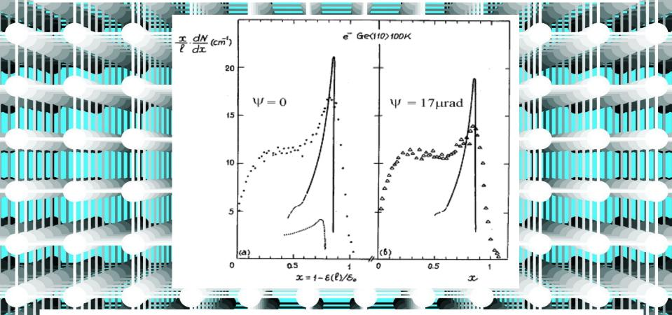
**Electron radiative loss spectrum** expressed in units of electron initial energy **150 GeV** at the angle of incidence  $\Psi$  = 0 and 17  $\mu$ rad on the Ge crystal plane <110> cooled to 100K. Dotted curve is calculated without taking into account the radiation cooling.
