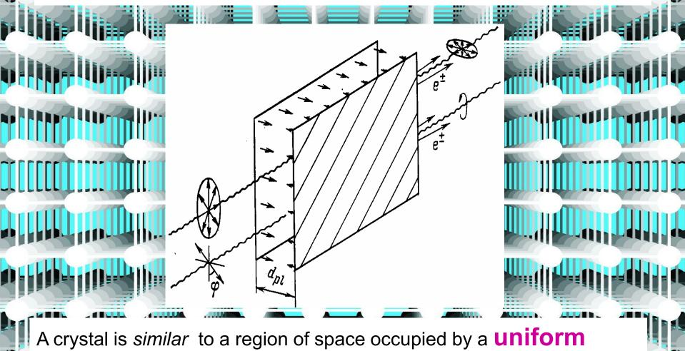
A crystal is similar to a region of space occupied by a **uniform** electric field and possesses the properties of **dichroism** and **birefringence** in very hard  $\gamma$  -region
