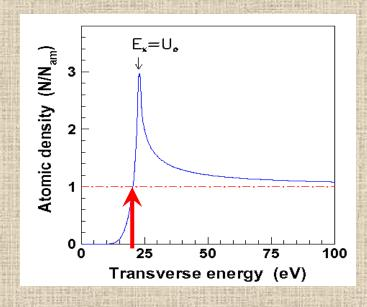
The dependence of the atomic density averaged along the particle trajectory in the (1 1 0) silicon crystal on the particle transverse energy.
