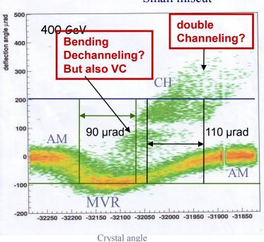
Yazynin simulation 8 Ideal strip crystals Si(111) "array" (L=2mm, R=10m, Alpha = 200 urad)
