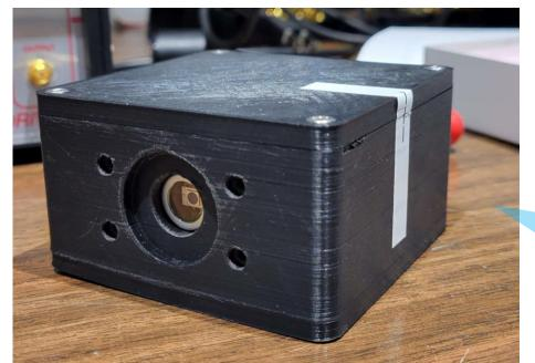
Switching to SiPM with increased linearity and is more robust
