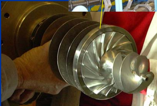
Impeller of the 1200 g/s centrifugal liquid helium pump
