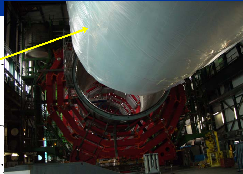
Solenoid coil during integration in cryostat
