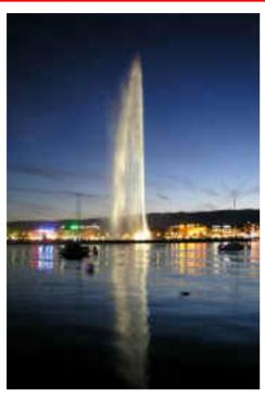
Water  $Jet \ height \sim 140 \ m$   $U = 56 \ m/s$   $D = 10 \ cm$   $Re_D \sim 5 \ x \ 10^6$   $Re_{\lambda} \ (@ \ x = 50D) \sim 1000 \ (rough \ estimation)$   $Power \ consumption = 10 \ MW$
