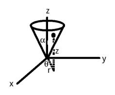
Consider a particle rolling due to gravity in a frictionless cone. The cone's opening angle α places a constraint on the coordinates tanα = r/z. We may write the Lagrangian in cylindrical coordinates
