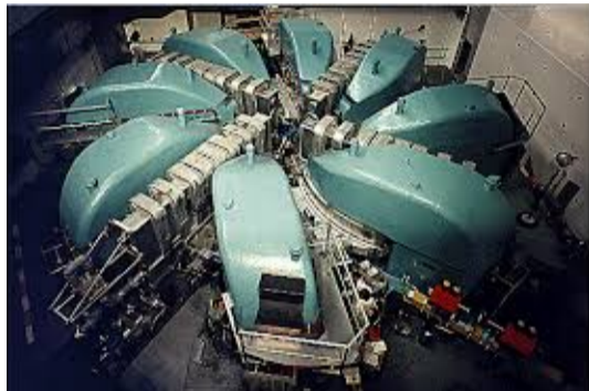
Figure: PSI cyclotron (250 MeV protons)
