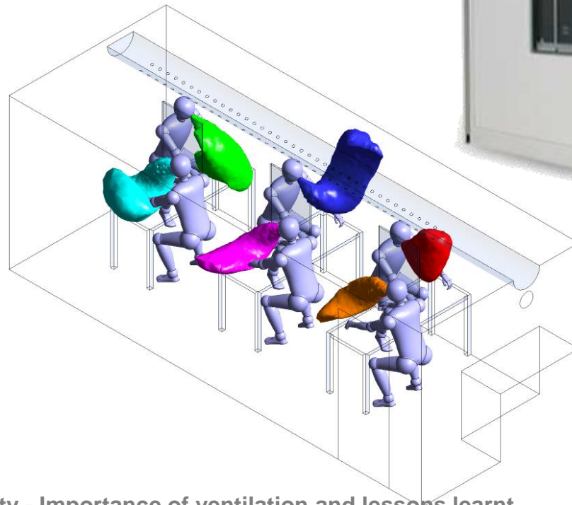
Contours of CO 2 concentration above 800 ppm (one color per occupant)
