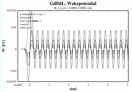
The amplitude of the wakepotentials grow linearly with the number of electrodes.
