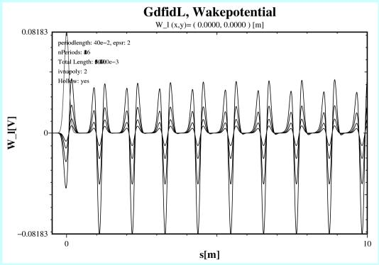
Two electrodes, 40cm, without dielectric Periodicity of 10/12.5 metres: twice the length of the electrodes times sqrt(epsr)
