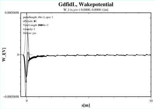
Two electrodes, 20cm, Epsr=2 Periodicity of 10/18 metres: twice the length of the electrodes times sqrt(epsr)
