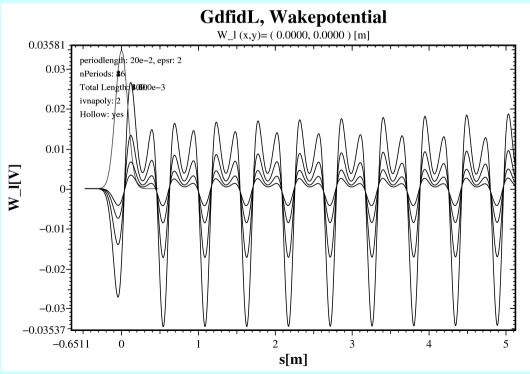
Two electrodes, 10cm, Epsr=2 Periodicity of 10/37 metres: twice the length of the electrodes times sqrt(epsr)
