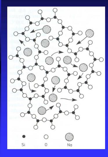
Schematic 2-dimensional representation of the Warren-Biscoe structure of alkali silicate glasses, showing the possibilities of localized and extended cationic motion within an anionic framework
