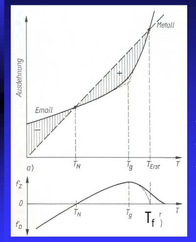
Development of tensions in the system metal/ enamel during cooling: + tensile stress - compressive stress T<sub>f</sub> = Point of fusion T<sub>g</sub> = Transformation temp. T<sub>N</sub> = Point of neutral stress
