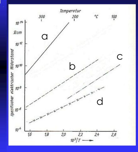
Temperature dependence of the specific electric resistance of different enamels:
