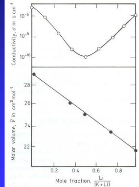
Substitution of  $Cs_2O$  in the glass 0,15 (Cs, M)<sub>2</sub>O \* 0,85 SiO<sub>2</sub> by different alkali oxides leads to a maximum for the electric resistance at approx. x= 0,5
