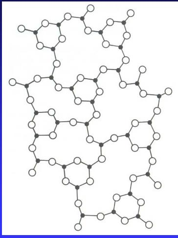
Schematic 2-dimensional representation of the Krogh-Moe structure of boric oxide glass with  $(B_3O_6)^{3-}$  boroxol groups
