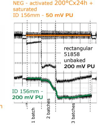
Activated NEG shows NO electron activity (note the different scales for the curves)
