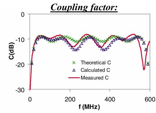
Theoretical C: according to the tabulated Zi values Calculated C: using Serenade simulations Measured C: using the VNA
