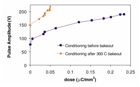
After a certain surface treatment (bake out or e- bombardment), the minimum pulse amplitude to trigger the multipacting is not achievable using the normal pulse amplifier.
