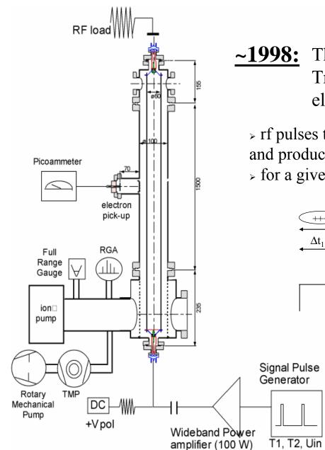
∼1998: The LHC/VAC Group at CERN installs a Traveling Wave (TW) chamber in its lab for electron cloud studies\*
