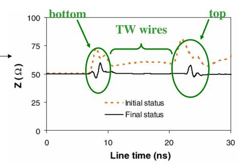
Careful redesign of adaptors between feedthroughs and wires
