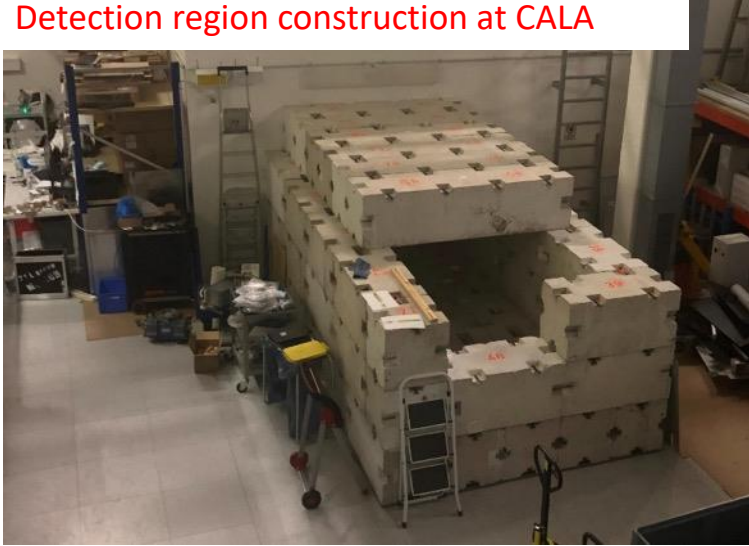
Lead and Cherenkov calorimeter assembly
