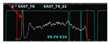
Longitudinal distribution visible on the wirescanners (position distribution via dispersion) and the spill (tune distribution via chromaticity)
