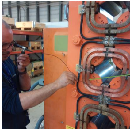
Inspections, measurements and simulations of the PSB Quadrupole Magnets
