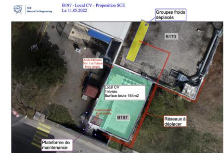
Fig. 4. SCE layout proposal: schematic view of the new Building at the top of the existing B. 197 and water-cooled chiller removed on the roof of B. 170
