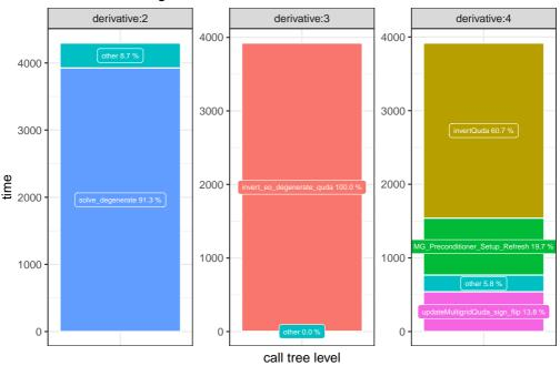
• Good: more than 90% of time spent in solver or unavoidable MG "overheads"
