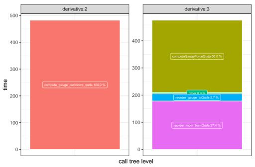
host-device transfers not a big deal even for gauge derivative, but we should move our field reordering completely to QUDA
