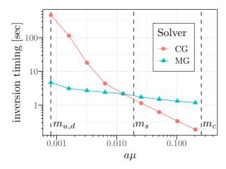
Comparison between MG-preconditioned-GCR and mixed-precision CG (GPU)
