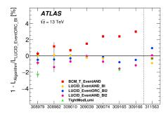
percentage deviation of the integrated luminosity with respect to the reference algorithm LUCID\_EventORC\_BI for all runs used in this analysis
