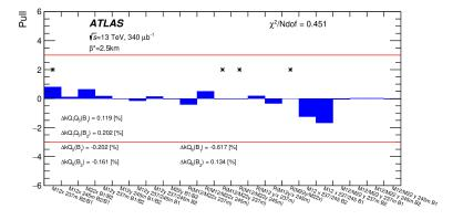
pulls from the effective beam optics fit of quadrupoles Q1, Q3, Q5 and Q6 to the ALFA constraints
