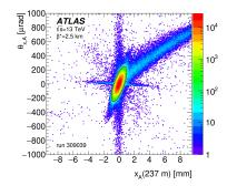
correlation between the coordinate and the local angle in the horizontal plane (after preselection and fiducial cuts, before acceptance and background rejection cuts)
