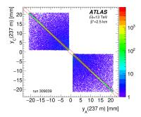
correlation of the *y* coordinate measured in the inner stations on the A-side and C-side (after preselection and fiducial cuts, before acceptance and background rejection)
