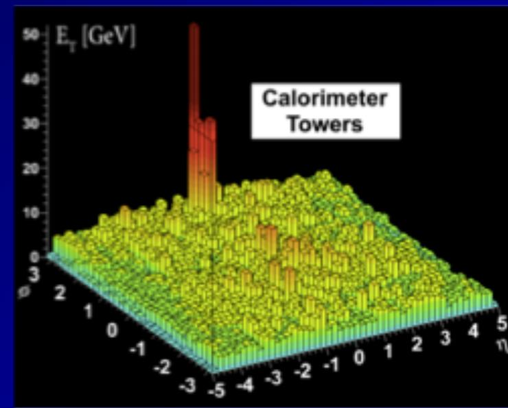
Jet energy as defined in the jet reconstruction algorithm with a jet cone  $R$
