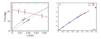
pure SU(3): linear behavior with small subleading term(s) the errors are hardly visible, V $\rightarrow$ 0 result is consistent with zero  $\chi_R^{-1}(V = \infty) = 0.0023(58)_{\text{stat}}(65)_{\text{sys}}$
