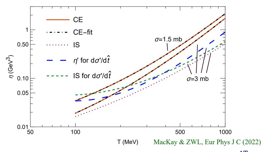
• We can use a  $h_2(w)$  fit function for forward scattering  $\eta^{CE} = \frac{4T}{5\sigma h_2(w)}$
