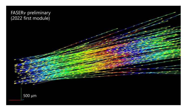
Reconstructed tracks (above ~1 GeV) in 1 mm  $\times$  1 mm  $\times$  20 emulsion films, which collected 0.5 fb<sup>-1</sup> of data.
