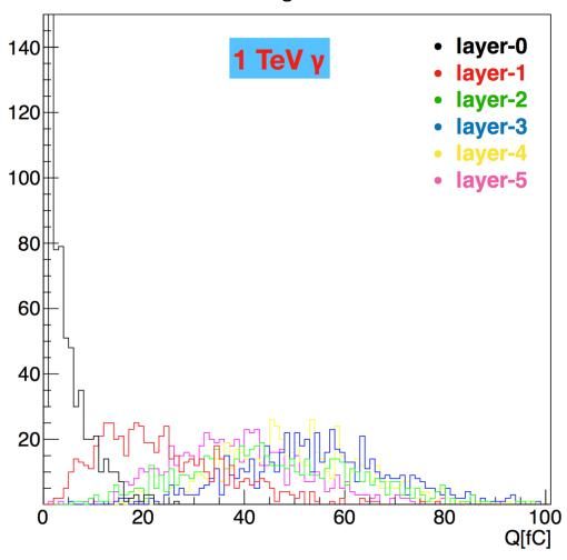
1 photon at E = 1TeV converting in the first layer
