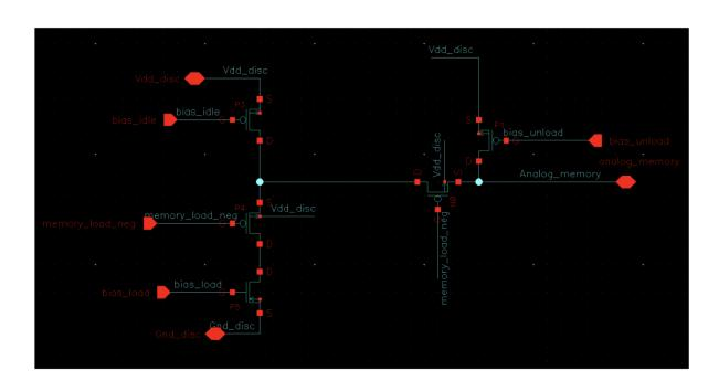
Current leakage even if the switch is opened. It takes 200 μs to degradate the memory value of 30 mV (= 1 bin of our ADC).
