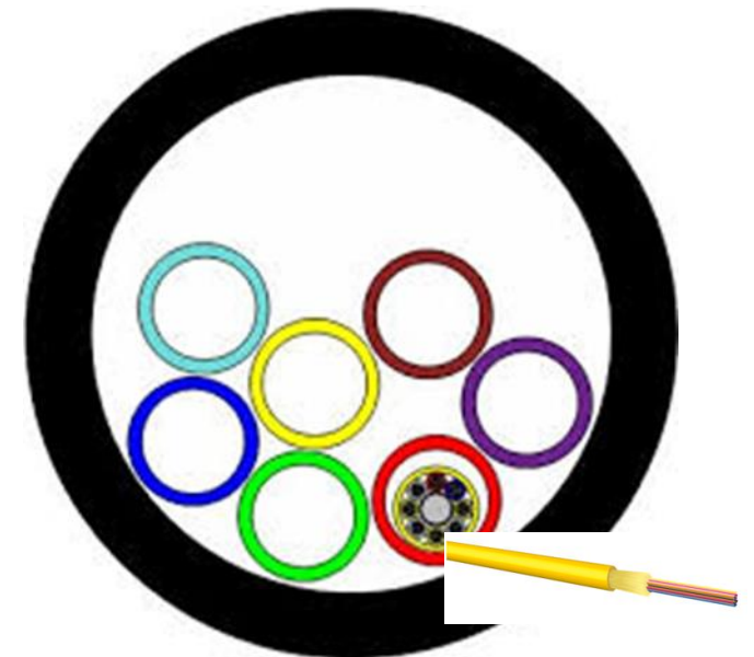
Microduct fibre cable
