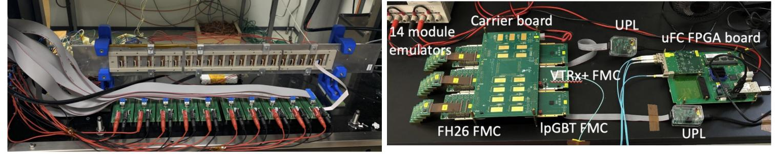
Ongoing preparation for full demonstrator with 55 full HGTD modules connected to prototype PEBs
