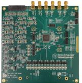
Provides **amplification** and **CR-(RC)<sup>2</sup> shaping** over two overlapping gain scales (High and Low), based on 130 nm CMOS technology, and will have 4-channel summing for hardware trigger.
