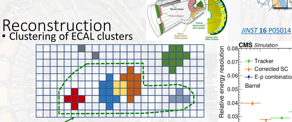
Refined superclusters use the information from the tracker, to be able to link bremsstrahlung emissions to missed ECAL deposits
