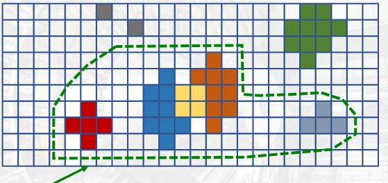
Refined superclusters use the information from the tracker, to be able to link bremsstrahlung emissions to missed ECAL deposits
