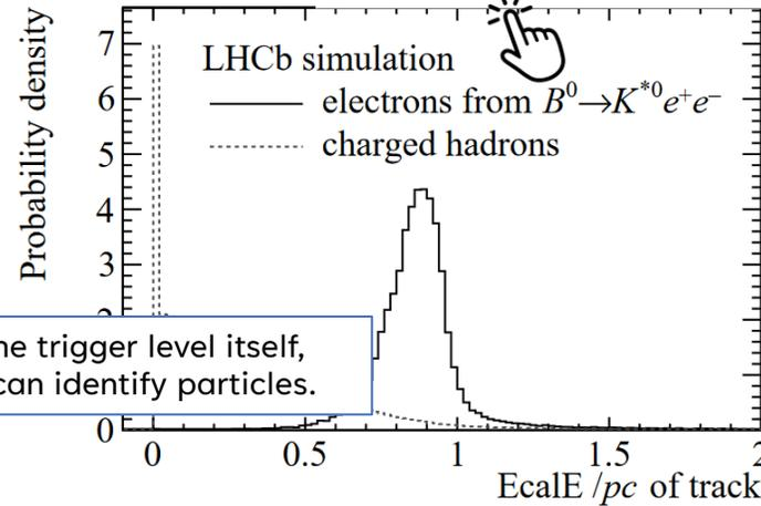
At the trigger level itself, we can identify particles.
