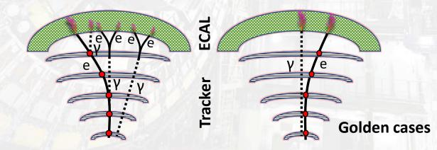
With bremsstrahlung and conversions
