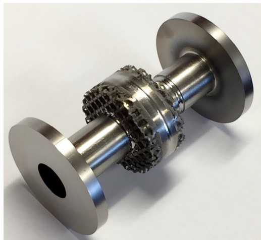
Figure 11: Photograph of the PBF-EB/M/Ni single-cell cavity.[32]
