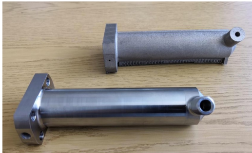
Figure 18: AM Ti-6Al-4V PROTAD target housings. [47]
