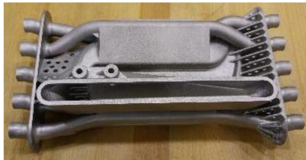
Figure 14: Additive manufactured lead-bismuth eutectic/water heat exchanger for LIEBE experiment. [38]
