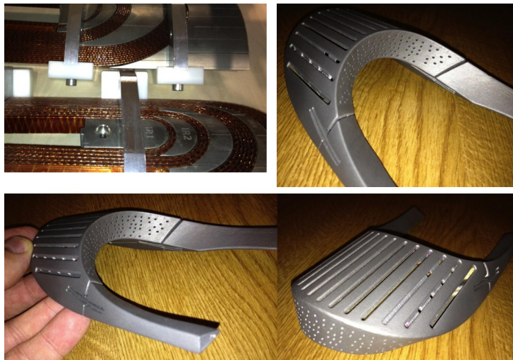
Figure 7: Additive manufactured Ti end spacers for MQXC. [21]
