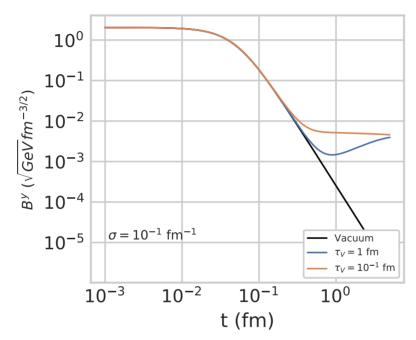
Longer τ<sub>v</sub> (the solid blue vs the solid orange line) means an incomplete response of the charge diffusion current and hence leads to faster decay of the magnetic field at early times.
