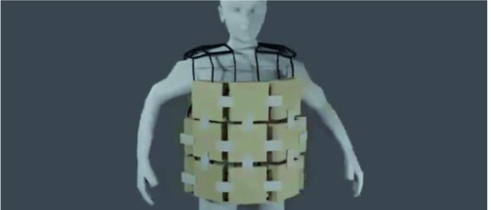
WPET - Wearable PET scanner jacket prototype
