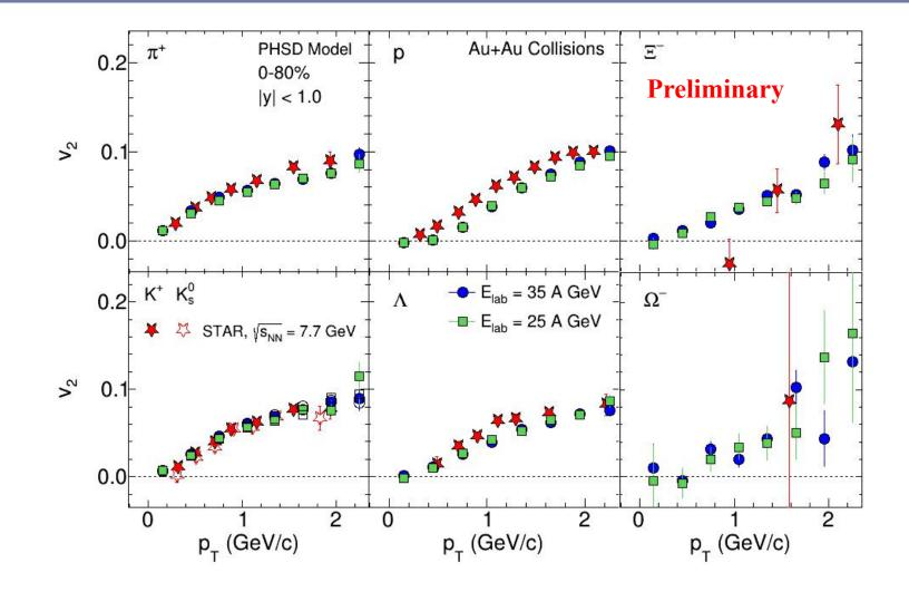
■ Identified hadron  $v_2$  ( $p_T$ ) in Au+Au collisions at  $E_{lab} = 35$  A and 25 A GeV from the PHSD model calculated with respect to the event plane and compared with the published STAR experimental results from Au+Au collisions at  $\sqrt{s_{NN}} = 7.7$  GeV.
