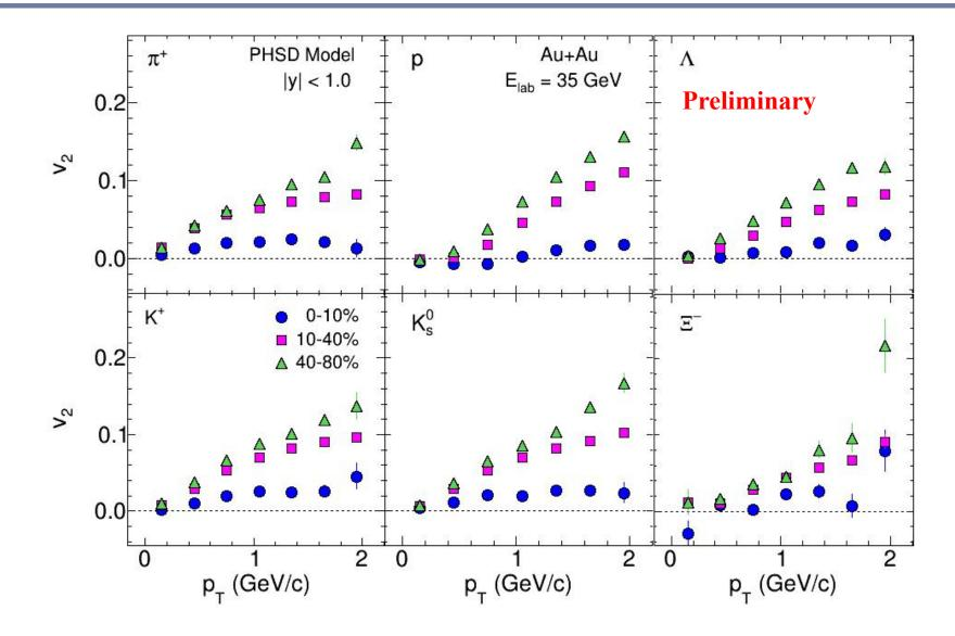
■ Identified hadron  $v_2$  ( $p_T$ ) in Au+Au collisions at  $E_{lab} = 35$  A GeV from the PHSD model for three different centrality intervals (0-10%, 10-40% and 40-80%).
