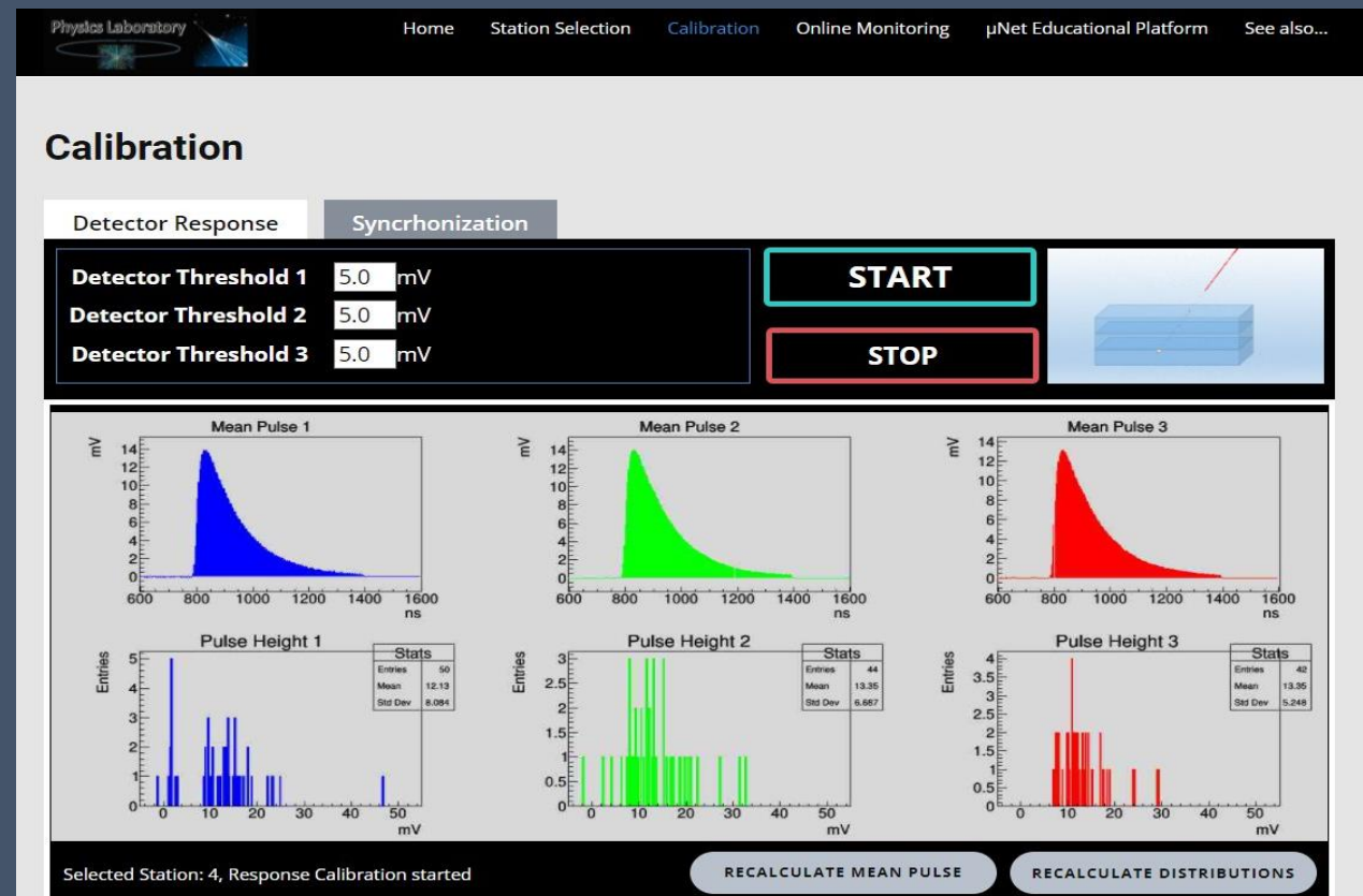
Means pulse and the pulse height distribution of each detector unit
