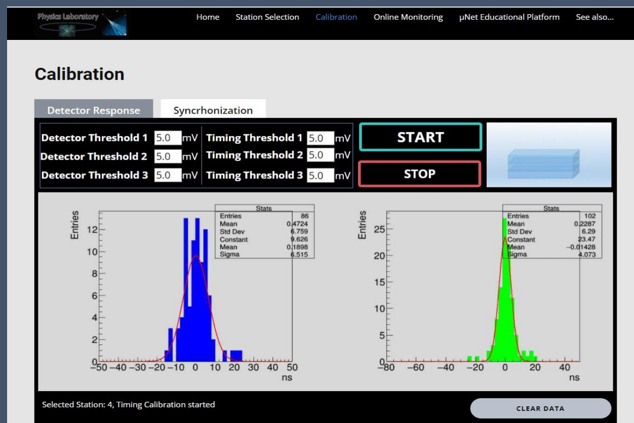
Time differences of the pulses for the two pairs of detectors
